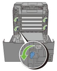
6 Hold the gray tabs, and then pull the PHD unit out of the printer.
